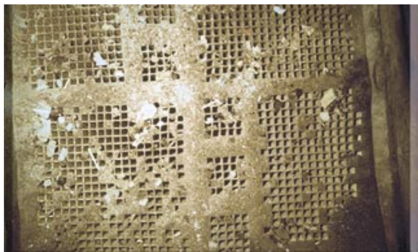
Plugging that may occur during normal operations of an SCR facility.
